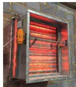
Damper Condition after 2 Hrs
