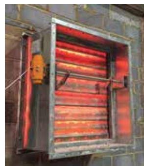
Damper Condition after 2 Hrs
