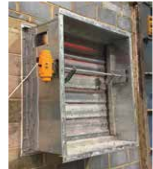
Damper Condition after 4 Hrs
