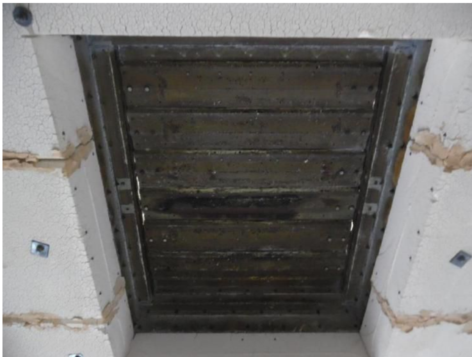
Photograph 3: Exposed face of the damper after test (closed position).
