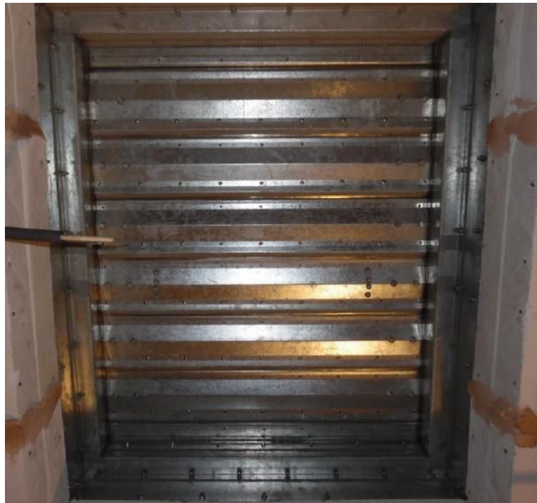
Photograph 2: Exposed face of the damper prior to test (closed position).
