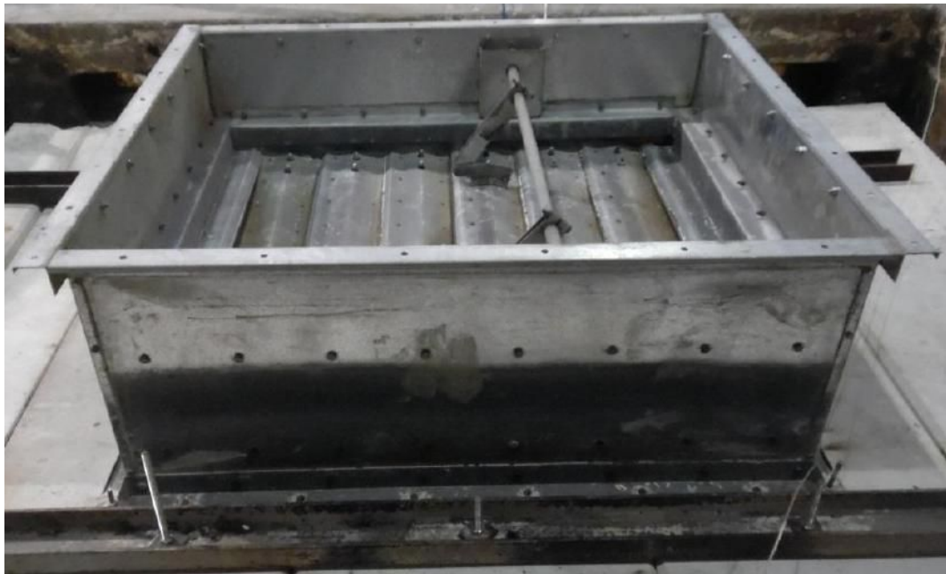
Photograph 5: Unexposed face of the damper after test (closed position).
