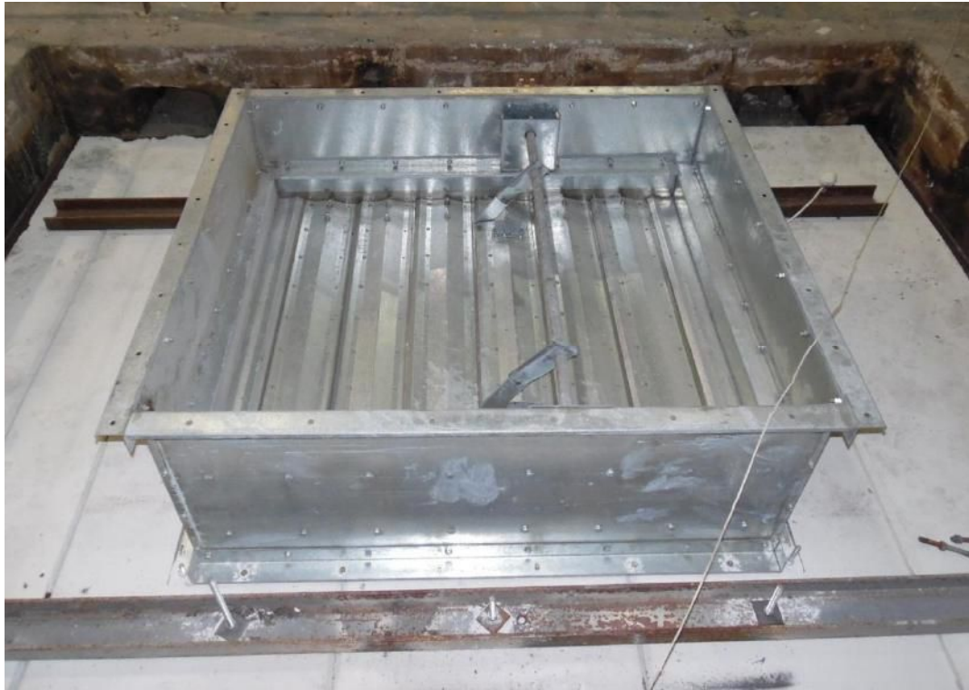
Photograph 4: Unexposed face of the damper prior to test (closed position).
