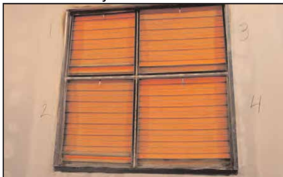
UL 555 Laboratory Tests Fire Damper After 2 hours - UL Laboratory
