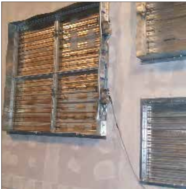
UL Fire tests - Damper after 3 hrs. Pictures courtesy UL-USA
